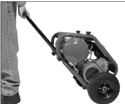
**IMPORTANT:** Only use pulling handle to pull unit, use the carrying handle to lift and carry unit.
