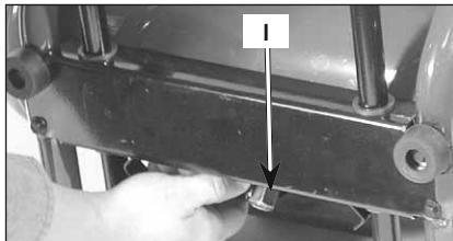
**Check Valve (L):** When the air compressor is operating, the check valve is "open", allowing compressed air to enter the air tank. When the air compressor reaches "cut-out" pressure, the check valve "closes", allowing air pressure to remain inside the air tank.
