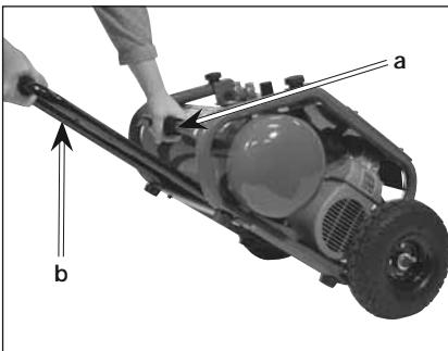
3. Pull unit as shown, do not push unit. **NOTE:** When transporting do not lift the unit to the point where it would tip over backwards.
